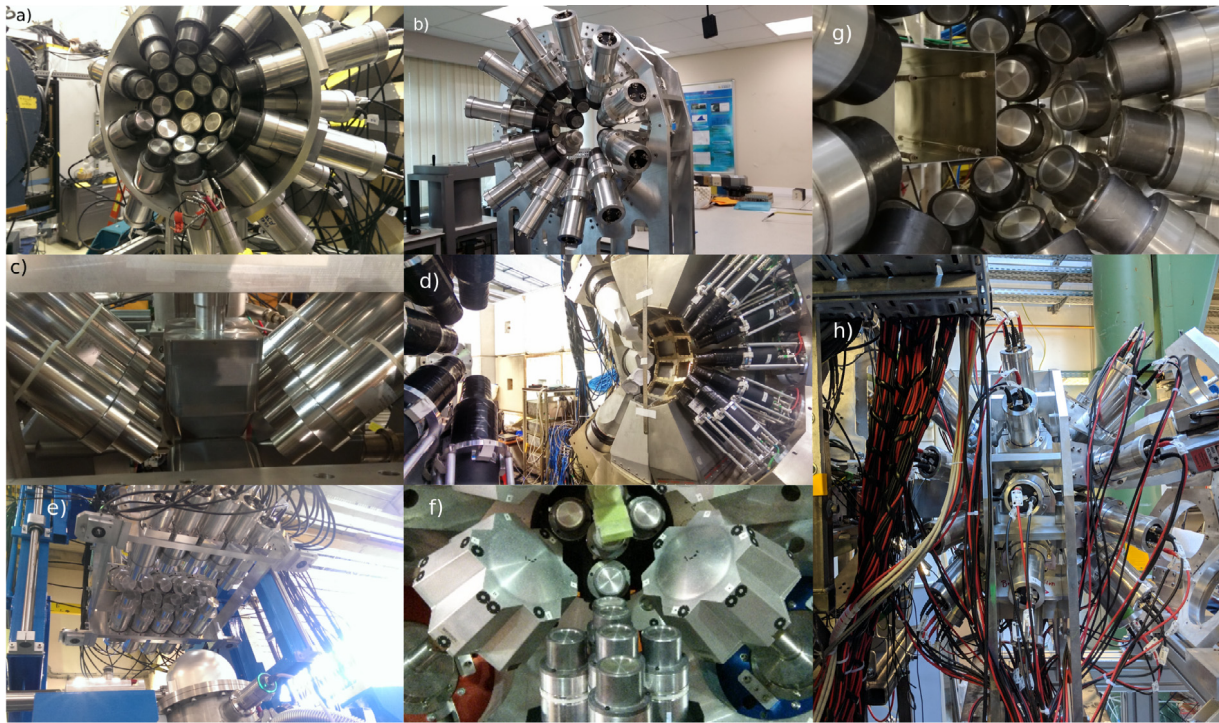
Fig. 14. (Colour online) Different setups in which the FATIMA detectors described in this paper have been mounted and used in experiments or tests. (a) At Argonne National Laboratory with half of the Gammasphere array. 25 detectors mounted in a hemisphere. (b) At the University of Surrey, some detectors are mounted on the DESPEC FATIMA frame in its core configuration with space for 36 detectors on three rings. (c) At GANIL at the LISE station together with HPGe Clover detectors. (d) At IPN Orsay during the \nu -Ball campaign 2017/2018. (e) At IPN Orsay for the Stella experiment. 36 detectors in a semi-cylindrical configuration. A manual lift system with counter-weights is used to allow access to the target chamber. (f) At RIKEN during the EURICA campaign. The detectors have been placed in free spaces in the array in clusters of six. (g) and (h) At GSI in the S4 cave in the configuration designed for use in the DESPEC station for FAIR (AIDA snout and rack to the left, beam from left to right).
