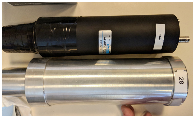
Fig. 3. (Colour online) Picture of the FATIMA detector parts. The PMT can be seen (black tube on top) with a \text{LaBr}_3(\text{Ce}) crystal taped on. This was how the detectors were mounted for the \nu -Ball experiment at IPN Orsay. The empty aluminium case of this detector can be seen below.
