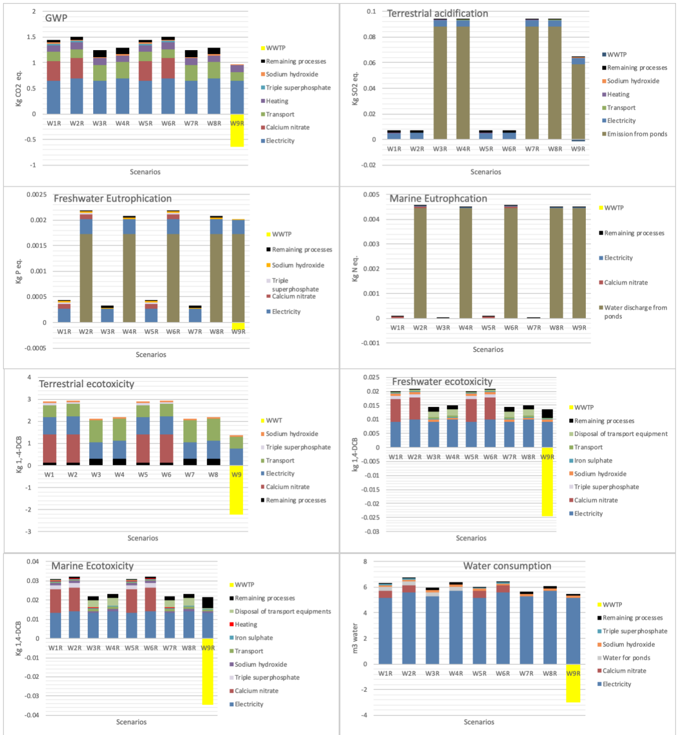
Figure 3. Contribution of the main inputs to the different impact categories. ReCiPe 2016 midpoint (H) V 1.03 method.
