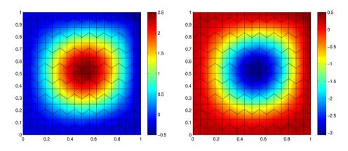
FIGURE 6. Test 3.  $u_1 := u_h$  obtained with  $\lambda = 55$ , f = 0 and  $\mathbf{u}^0(x, y) = (\frac{1}{4}(yx^2+1), \frac{1}{4}(yx^2+1))$ (*left*).  $u_2 := u_h$  obtained with  $\lambda = 55$ , f = 0 and  $\mathbf{u}^0(x, y) = -(\frac{1}{4}(yx^2+1), \frac{1}{4}(yx^2+1))$  (*right*).
