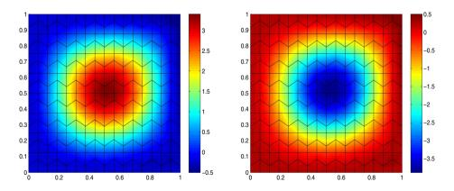
FIGURE 7. Test 3.  $u_1 := u_h$  obtained with  $\lambda = 60$ , f = 0 and  $\mathbf{u}^0(x, y) = (\frac{1}{4}(yx^2+1), \frac{1}{4}(yx^2+1))$ (*left*).  $u_2 := u_h$  obtained with  $\lambda = 60$ , f = 0 and  $\mathbf{u}^0(x, y) = -(\frac{1}{4}(yx^2+1), \frac{1}{4}(yx^2+1))$  (*right*).
