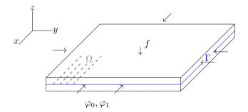
FIGURE 1. Plate subject to transversal and lateral forces  $f \in L^2(\Omega)$  and  $(\varphi_0, \varphi_1) \in H^{5/2}(\Gamma) \times H^{3/2}(\Gamma)$ , respectively.
