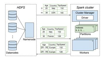
Fig. 2. Architecture and working of the distributed anonymization system
