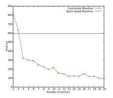
Fig. 3. Execution times of the centralized version and distributed version varying the number of workers
