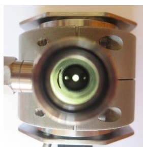
Figure 5. Upper view of the opened cell, showing the three holes that connect the stirred part of the cell with that where the IR beam passes through and the side port connecting the cell body to the gas valve and pressure gauge. A light was inserted in the lower compartment to improve the contrast in the picture.
