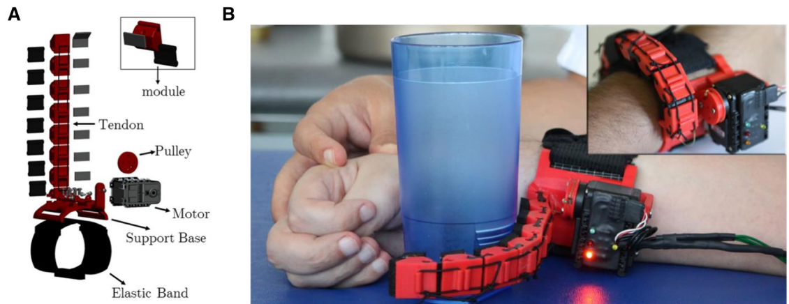
Figure 1. The Soft Sixth Finger. (A) The SSF has a modular structure. Each module consists of a rigid ABS part and a soft Polyurethane part that acts like a soft joint. The finger is actuated by a tendon-driven system with a single motor. (B) Upper right corner: the finger can be worn at the forearm and can be wrapped around the wrist when not used. When in use, the SSF acts as a gripper with the rest of the hand (in this case a paretic hand is shown). [Original photographs taken by Gionata Salvetti].
