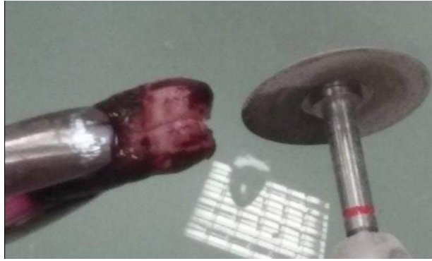
Figure 19 Sectioning of a sample using a steel disk.
