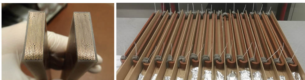
Figure 3.3: Cross-section of a superconducting coil of the MCTXF magnet to evaluate the stacking factor of the wires in the winding (left). The coils are produced in series and have to satisfy the geometrical quality criteria to be used for the assembling in the magnet (right)
