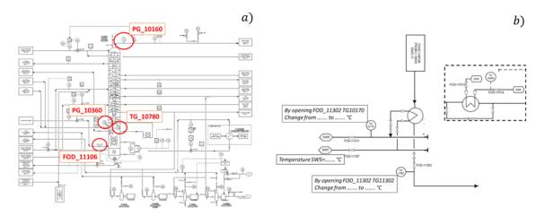
Figure 3: PID scheme for the exercises ""Distillation Column Operation" and "Sequential Patrol Heat Exchanger".
