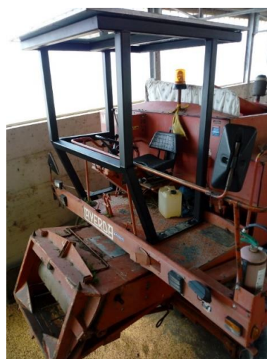
Figure 15. Physical model of TOPS retrofitted on the combine harvester.
