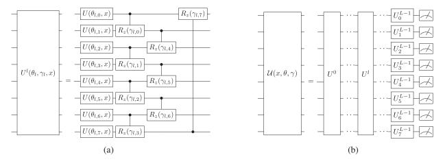
FIG. 3. On the left we show an example of one layer architecture. On the right we present the scheme of a full Ansatz circuit including 8 qubits and entangling gates. The  $U^{l}(\theta_{l}, \gamma_{l}, x)$  from the left figure enters the full ansatz as  $U^{l}$ . Note that the last layer does not have any entangling gate.
