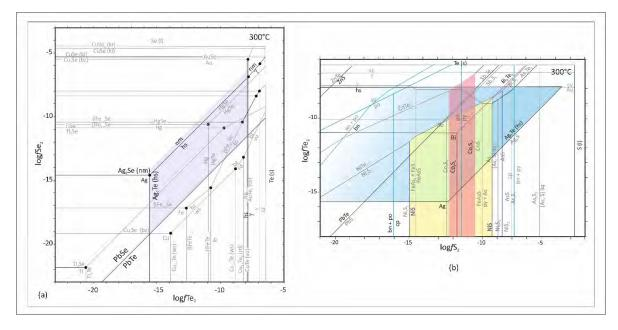
**Figure 17.** Phase relations for selenides and tellurides (a) and for selenides, tellurides and sulfides (b) in function of  $\log f$ Te<sub>2</sub>, fSe<sub>2</sub> and fS<sub>2</sub> at 300 °C by [57,112–115]. The colored areas represent stability fields for the selenide, telluride and Co–Ni sulfide phases observed in the Piazza mineralization.
