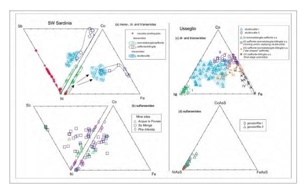
**Figure 6.** Plots of the data of arsenides and sulfarsenides (atomic%). (a,b) ternary diagrams comparing Ni, Co, Fe, and Sb components for mono-, di-, and triarsenides and for sulfarsenides–sulfantimonides in the SW Sardinian vein system; (c,d) ternary diagrams comparing Ni, Co, and Fe components for diand triarsenides and for sulfarsenides in the Usseglio vein system.
