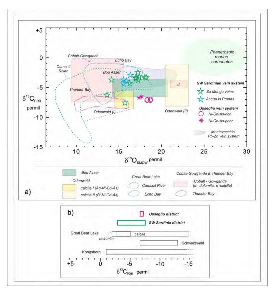
**Figure 16.** Stable isotope composition of ore-related carbonates. (a) Carbon and oxygen and (b) carbon-only isotopic composition of Fe carbonates from the SW Sardinian and Usseglio vein systems and comparison with isotopic data from the Montevecchio Zn–Pb vein system [30] and from several Co–Ni-rich, five element vein-type ore deposits world-wide [1,7,78–84]. Compositional field for Phanerozoic marine limestones after [78].
