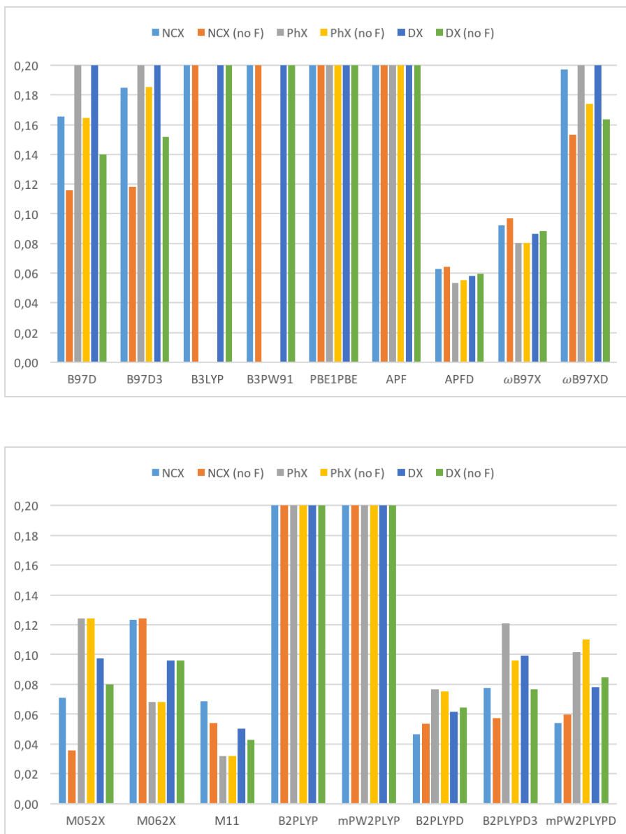
Figure 4. Mean absolute relative errors on topological properties at BCPs, \langle \mathcal{E} \rangle_{\text{QTAIM}} , for the different DFT functionals. Color of the bars means: Light blue, NCX/ \pi ; Orange, NCX/ \pi excluding fluorine; Gray, PhX/ \pi ; Yellow, PhX/ \pi excluding fluorine; Blue, NCX/ \pi and PhX/ \pi ;
