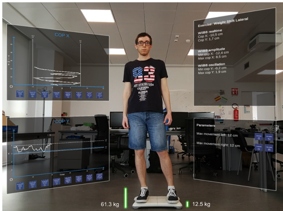
Figure 7.3: Mirarts main view. On the left, it is possible to see the graphs showing the trend of the CoP during the execution of the exercise. On the right, in addition to a series of summary metrics (top box), it is possible to change in real-time the main parameters of the exercise (bottom box).
