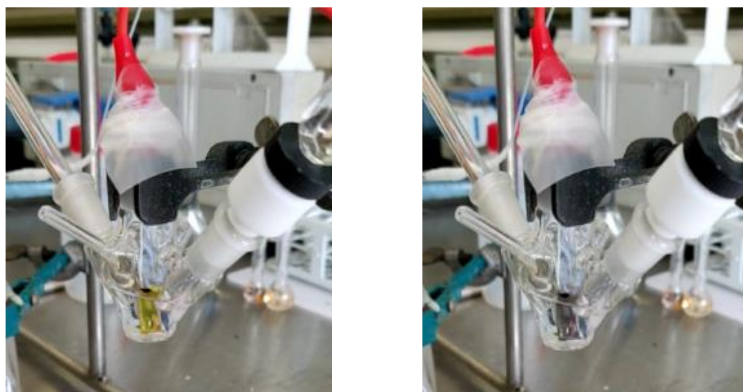
Figure 56: Film of 98c in neutral (yellow, left) and in oxidative (blue, right) phase.
