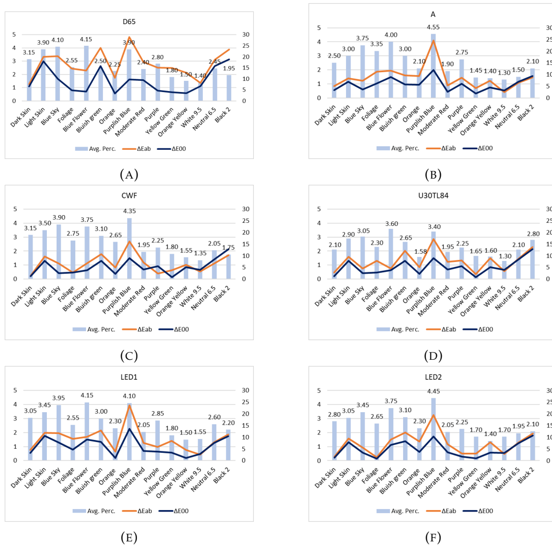
FIGURE 3.6: Representation of the average perceived color difference compared with the measured values of \Delta E and \Delta E_{00} for the light sources: D65 (Figure 3.6a), A (Figure 3.6b), CWF (Figure 3.6c), U30TL84 (Figure 3.6d), LED1 (Figure 3.6e) and LED2 (Figure 3.6f).
