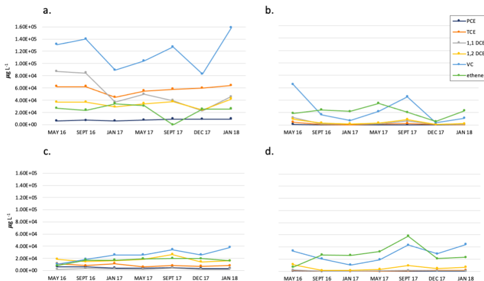
Figure 8 Chloroethenes concentrations during 20 months in the four piezometers: Pz13 (a), Pz10 (b), Pz16 (c) and Pz3 (d).
