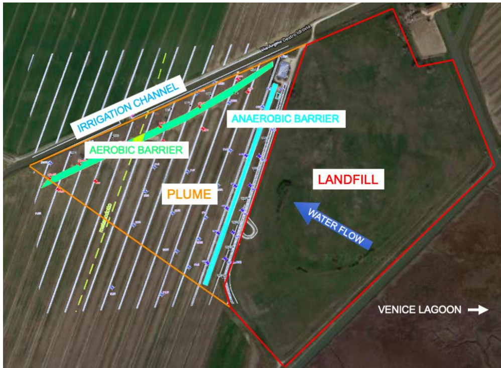
Figure 11 Setup map of two sequenced multi permeable reactive bio barriers in the site for the bioremediation of the aquifer
