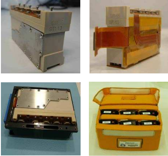
Fig. 1. Top left) SPHINX EU. Each EU is composed of a brick of biological compatible plastic (PEEK®) where five cylinders, a culture chamber (CC) and connecting channels are machined. Five small valves separate the different fluids and the CC. Each cylinder has a piston for the fluid injection into the CC; once the piston is released by a preloaded spring, the fluid contained into the cylinder flows into the CC and the waste medium is recovered behind the activated piston and suitably preserved with a protease inhibitor cocktail. Top right) SPHINX EU and integrated electronics. Bottom left) SPHINX integrated into the KIC-SL experiment container (EC). Bottom right) SPHINX EH in the soft pouch.
