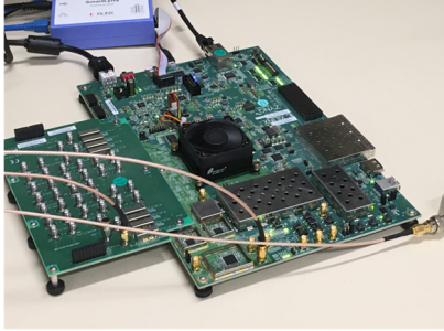
Xilinx ZCU111 RFSoc FPGA digitizer/channelizer
