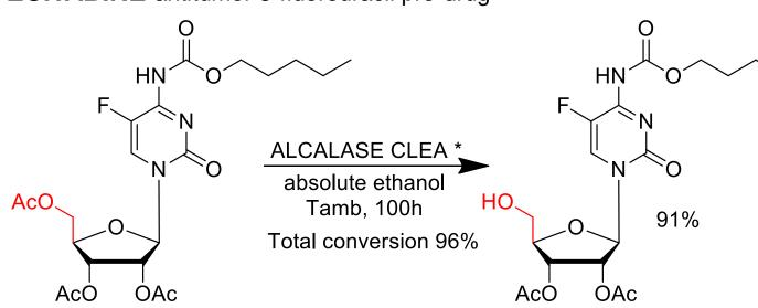
With an enzyme mediated REGIOSELECTIVE ALCOHOLYSIS only the primary alcool was deprotected in order to have the proper modified sugar moiety.
