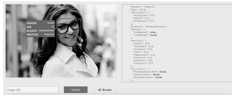
Figure 1. An example of emotion detection with API.
