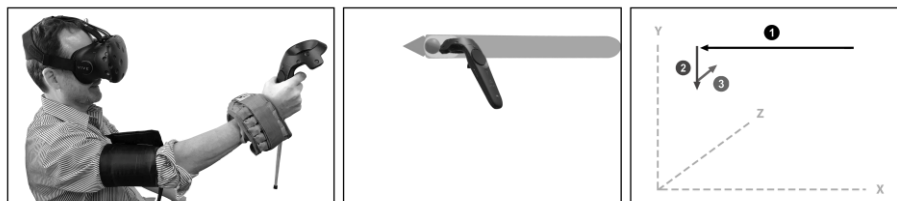
Figure 1. Left: VR headset and hand controller, sphygmomanometer cuff and wrist weight. Center: View seen in VR, showing a leader ball prescribing Segment 1 of the movement path in the Follow-the-Leader Task. Right: First three (of 21) segments in the predefined movement path of the leader ball (Phase II).
