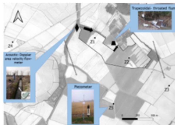
Fig. 1 Study area and position of the monitoring devices. Piezometers (from Z1 to Z5) are shown by black dots, the acoustic-Doppler inflow-meter by a diamond, and outflow flumes by a trapezoid. The main groundwater flow direction is shown by dashed arrows, while surface water flow direction by black arrows.
