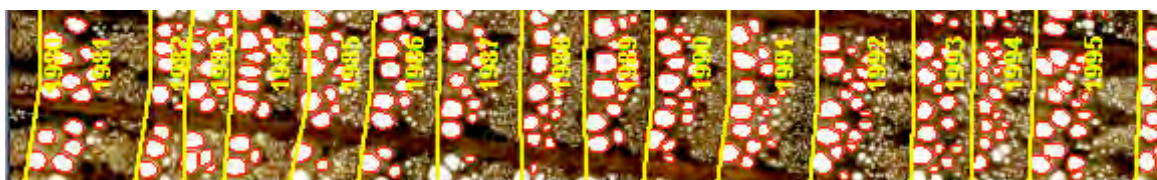
Fig. 1 - Example of earlywood vessel extraction and tree-ring detection by image analysis on oak wood
