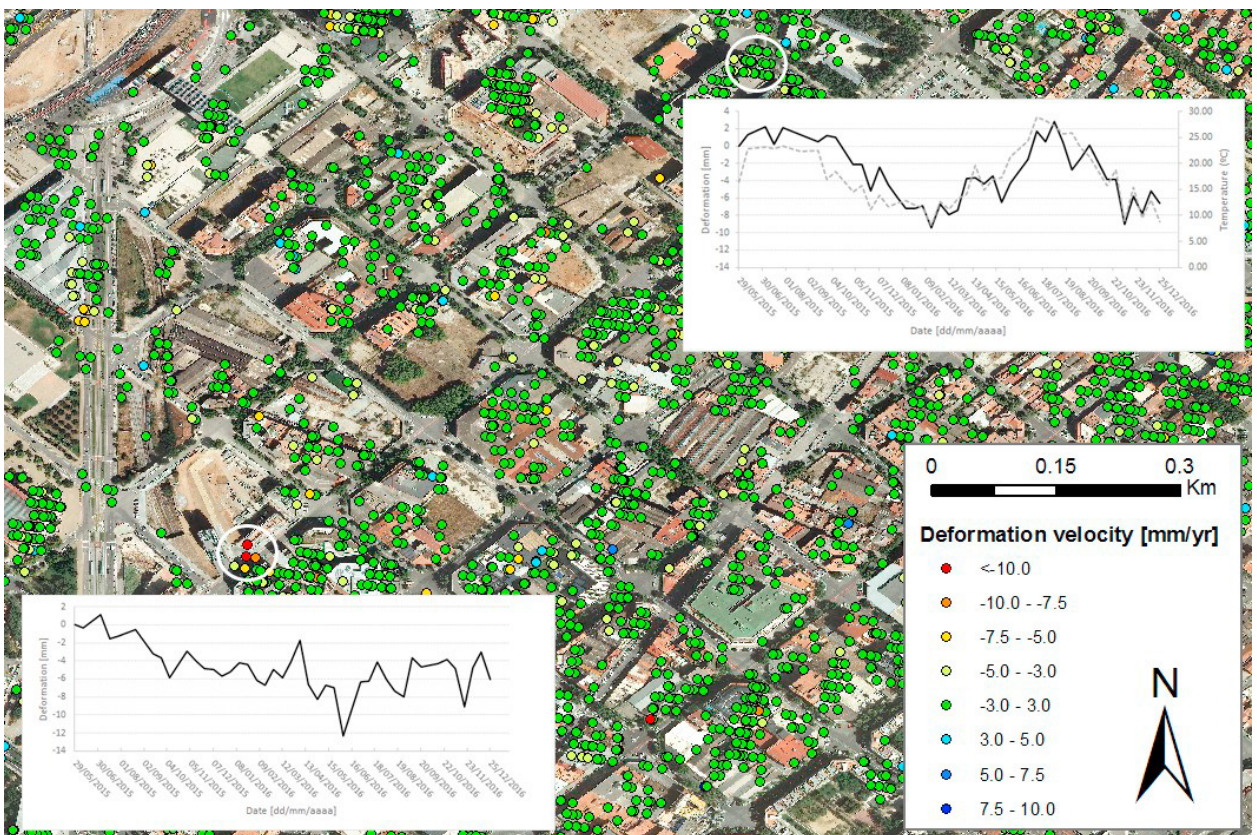
Fig. 3. Deformation velocity map displaying a portion of the area of interest. The time series of two Persistent Scatterers are shown.
