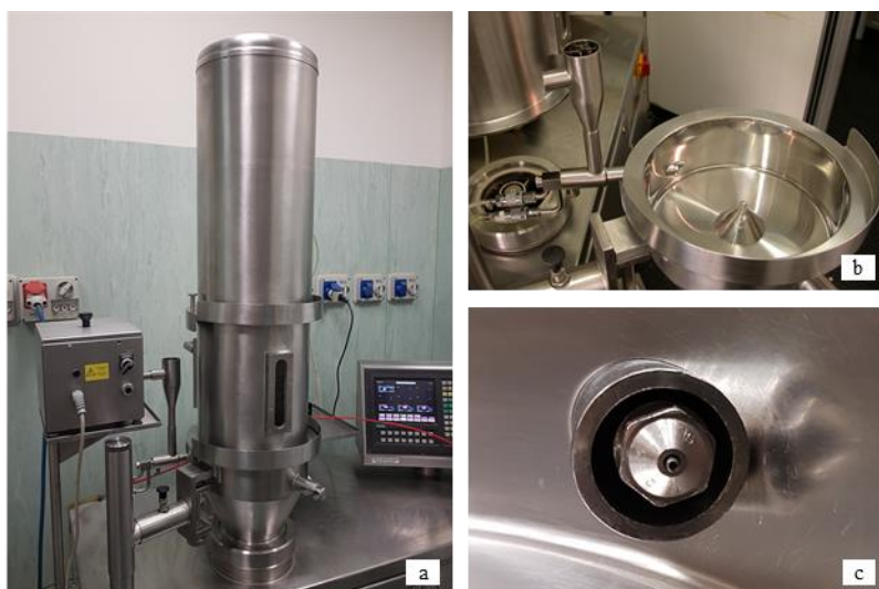
Figure 1. GPCG-1 fluid bed apparatus with rotor insert (a), open rotor insert equipped with powder feeder (b) and three-way nozzle with peripheral port for powder dosing (c).
