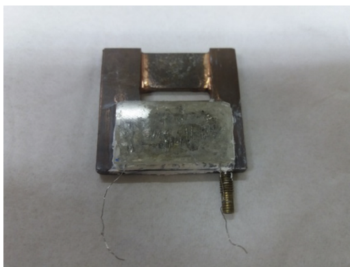
FIG. 3. Copper cooler designed to control the temperature of the nitrogen gas located above the sample. The picture shows a copper tube for the inlet of cold nitrogen vapor and two nichrome wires which are coiled around a mica sheet for heating the copper cooler. The terminals of the nichrome wires are connected to the PID Controller (G, Fig. 2) by crocodile clips, which can be observed in Fig. 1(b).
