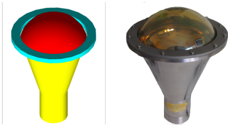
FIG. 4. Comparison between the schematization of the outer detector PMT in the simulation (left) and the real object (right).
