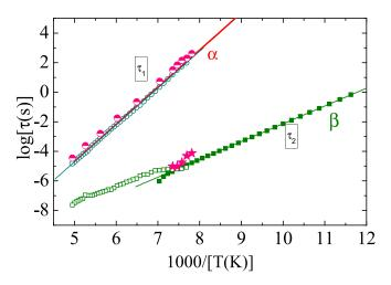
FIG. 4. Relaxation times as a function of reciprocal of temperature for the different relaxation processes. Open circles:  $\alpha$  relaxation (experimental values); open squares:  $\beta$  relaxation (calculated values according to the CM model (Refs. [15,16]); full green squares:  $\beta$ relaxation (experimental values). Pink symbols are calculated according to our proposed theoretical model (see Table I): Full-empty circles for  $\alpha$  relaxation and stars for  $\beta$  relaxation.
