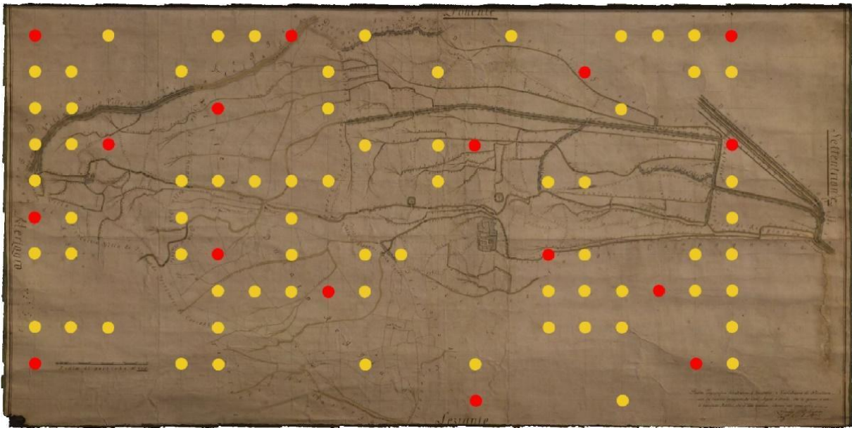
Figure 4. Cartographic grid points used as Ground Control Points (GCPs) (69 points marked in yellow) and Checkpoints (CPs) (16 points marked in red).
