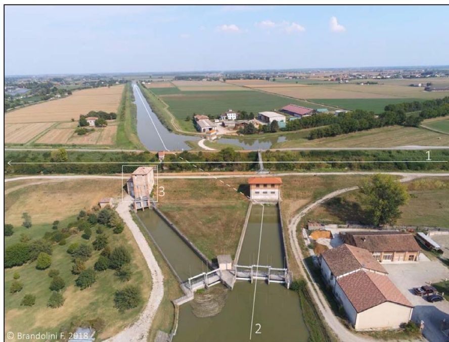
Figure 15. The crossing between the Crostolo River (1) with the Parmigiana Canal (2) in the modern completely drained countryside. The white square highlights the 17th century AD structure of the Botte Bentivoglio hydraulic device (3).
