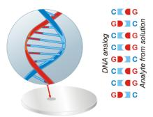
We devised and fabricated a chemosensor for selective determination of genetically relevant 5'-GCGGCGGC-3' (G-guanine, C-cytosine) oligonucleotide. Toward that, we simultaneously synthesized electrochemically and deposited on a Pt electrode a sequence-defined *octakis*(2,2'bithien-5-yl) polymerized film of a DNA hybridizing probe.<sup>1</sup> For that purpose, we used both an approach of macromolecular imprinting in a polymer and a peptide
