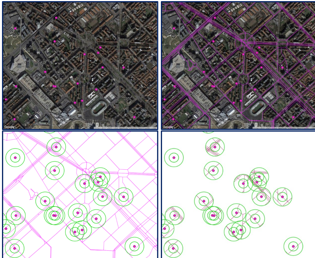
Figure 23. GIS visualization of the intersection procedure between buffers and road layer used in the LUR selection process of explanatory variables
