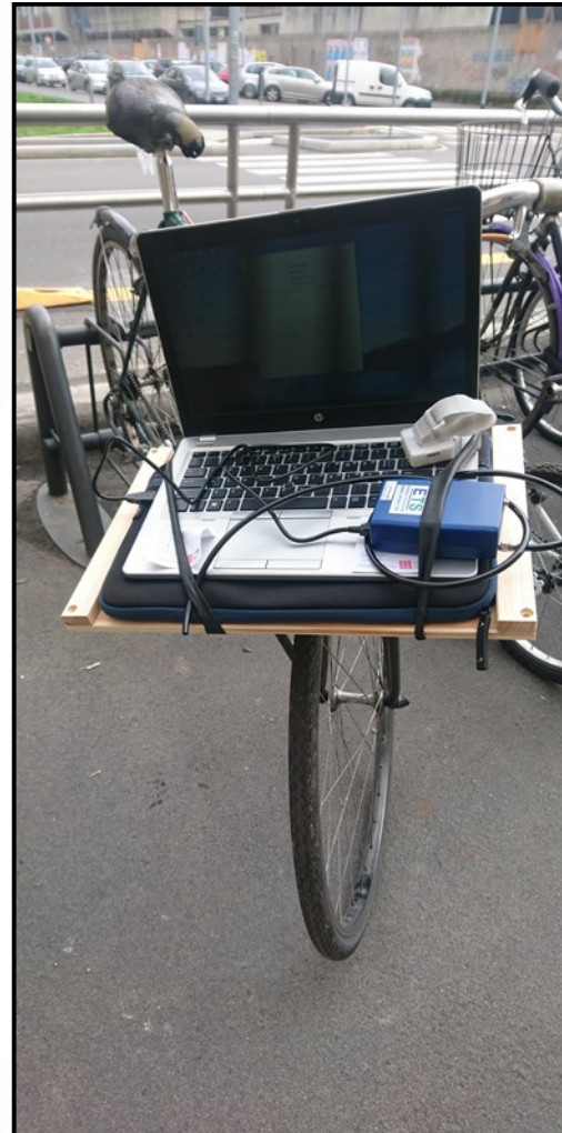
Figure 30. On the left, the identikit of BC and other pollutants presented as characters is reported. In the middle a bicycle equipped with a laptop and a microaethalometer AE51. The bicycle was used for the online measurements in the neighbourhood. On the top-right a moment during which children were asked to say if there was normal, high or very high level of BC according to the location and their perceives; on the mid-right one of the maps developed using the data collected during each neighbourhood measurements; at the bottom-right of the figure. a moment during which children were asked to figure out the place according to the level of BC is reported.
