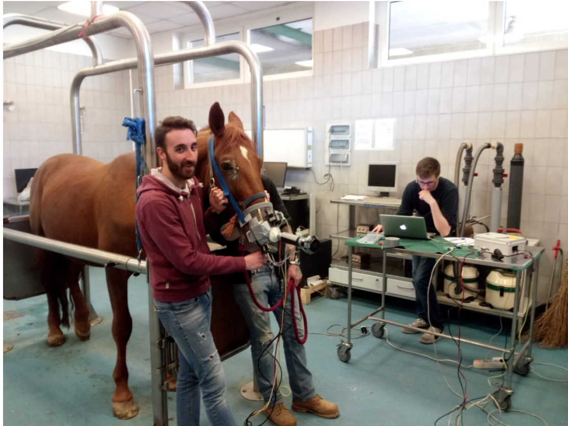
Figure 5. A horse undergoing FOT measurement. Notice the FOT device attached to the airmask.
