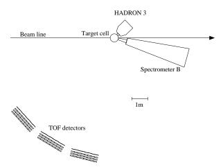
Fig. 3. Diagram of the detector set-up for the calibration runs using the  $^{2}$ H cryogenic target.
