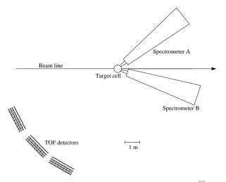
Fig. 2. Diagram of the detector set-up for the  ${}^{16}O(e,e'pn)$  experiment using the waterfall target.
