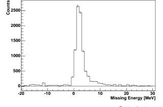
Fig. 7. Missing energy distribution for the  ${}^{2}H(e,e'pn)$  reaction. The peak has a mean of 2.1 MeV and the resolution amounts to 3.0 MeV (FWHM).
