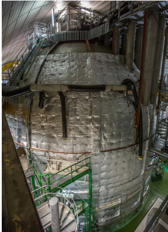
Figure 6.5: Photography of the Borexino detector, showing the external layer of mineral wool applied to improve the thermal insulation.
