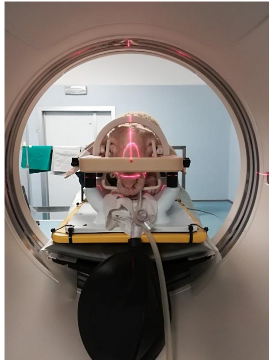
Figure 4: in-vivo clinical setting of live ovine model with the head frame system during a CT acquisition
