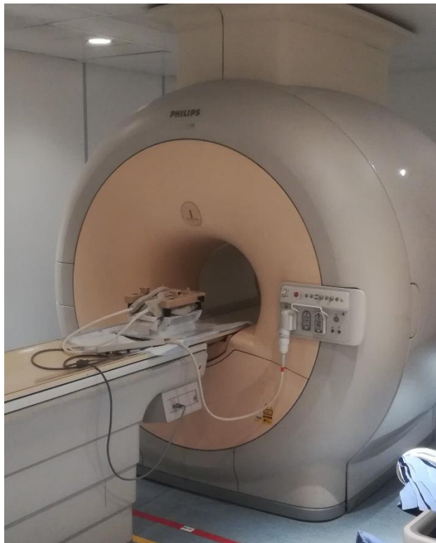
Figure 7: MR test setup with the Head Frame placed inside the bore of the machine
