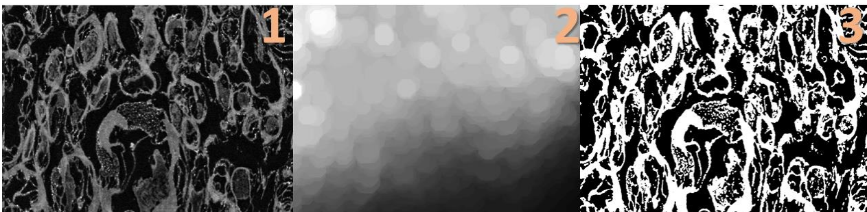
Figure 3 After filtering salt and pepper noise (1) and subtracting the unevenly illuminated background (2) the image is binarized (3).
