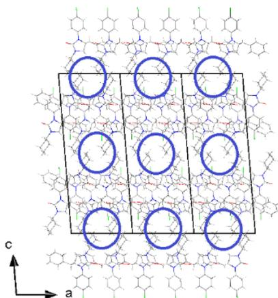
**Figure S6.** Crystal packing of **3ea** viewed down the *b* axis. The void space among cyclohexyl units, potentially able to allocate solvents, is highlighted as blue circles.
