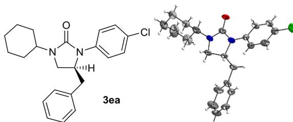
Figure 4. Left: Molecular structure of the *S*-enantiomer of the compound **3ea**, as determined by single crystal X-ray diffraction. Right: ORTEP scheme showing the corresponding in-crystal molecular conformation of (*S*)-**3ea** at r.t. Thermal ellipsoids are drawn at the at the 25 % probability level. C: gray; H: white; O: red; N: blue; Cl: green.
