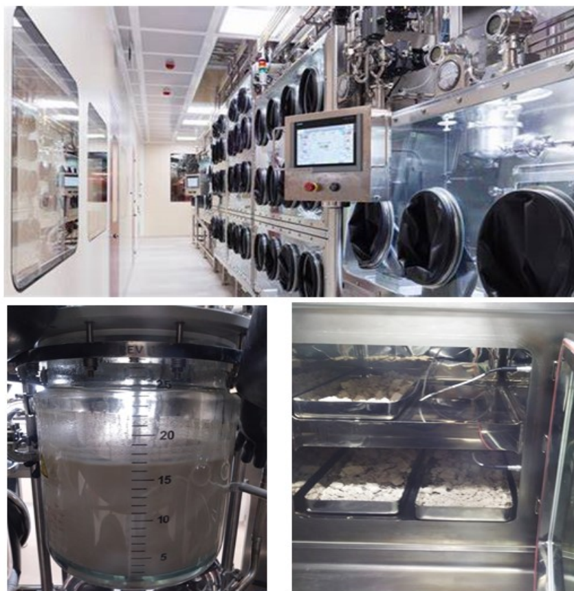
Figure 3.3. High containment Kilo-Lab (25 L vessel and oven).
