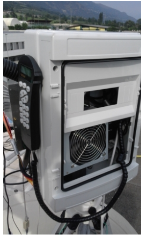
Figure 2.13. The box containing ARBOL's power supply and the motor controls
