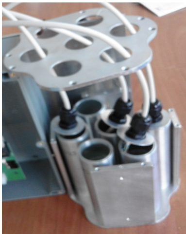
Figure 2.2. ARBOL during maintenance. An unscrewed flange can be appreciated
