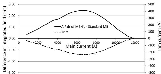
Fig. 7. The solid line shows the difference in integrated field between a pair of MBHs and an MB, both delivering 119 T·m at 11.85 kA. The dotted line shows the trim current needed to correct the difference at currents below 11.85 kA.
