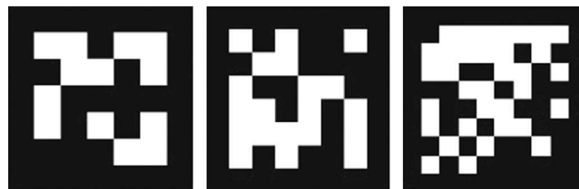
FIGURE 7 THREE EXAMPLES OF ARUCO FIDUCIAL MARKERS MADE (FROM LEFT TO RIGHT) OF 5 \times 5 , 6 \times 6 , 8 \times 8 BITS
