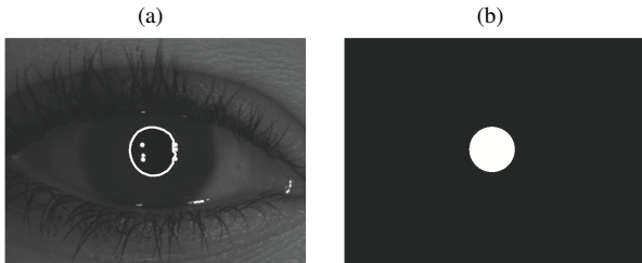
Fig. 6. Example of the results obtained using the proposed algorithm for the estimation of the internal iris boundary: (a) the identified pupil area and (b) the corresponding binary mask obtained from the refined boundary points v_B .
