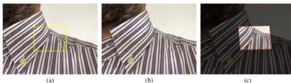
Figure 7. Mobile application: tracking small movements of the mobile device via the built-in front camera. (a): reference frame, with a yellow rectangle indicating the central portion of the frame whose motion is actually tracked. (b): a later frame, where the user roughly appears to have moved to the right (actually, it is the mobile device that is moving while the user plays the virtual flute, and the motion is not a pure translation). (c): the algorithm computes the motion, thus allowing to project the central portion of (a) onto (b) and, ultimately, to determine which virtual pipe is below the mouth of the user.
