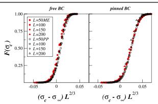
FIG. 2 (color online). Cumulative distributions of yield stress for free and pinned boundary conditions for ME and PP. The distributions can all be collapsed with the same exponent, related to  $\theta = 1/3$ .
