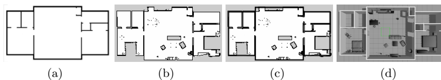
Fig. 1: An example of floor plan (1a), a map built by the robot (1b), an overlay of the floor plan on the map (1c), and the environment simulated in Gazebo (1d).
