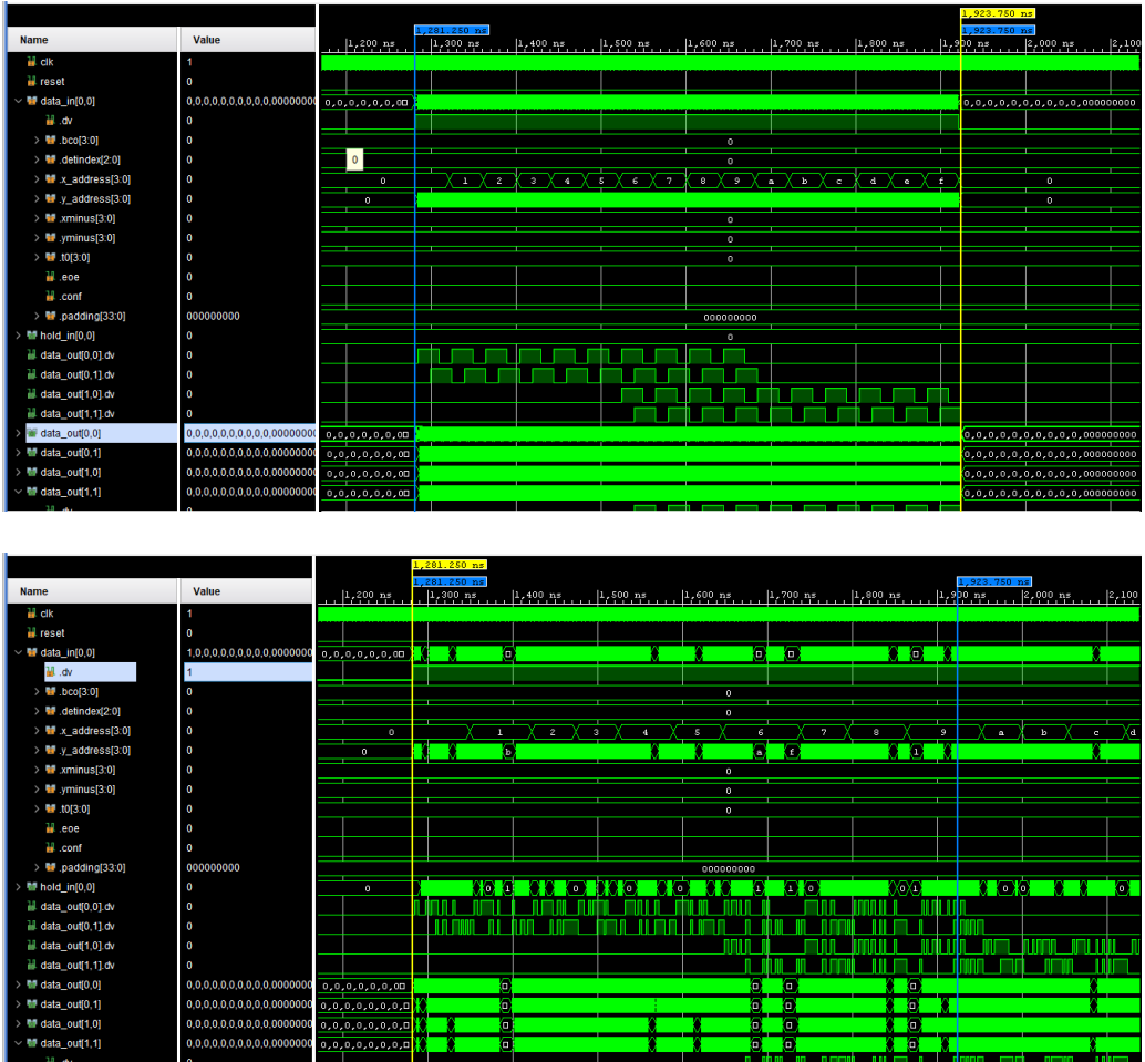
Figure 5.15: Testbench of the N-Way Dispatcher. In the top picture a sequence of 256 data is provided to the data_in port and no hold is provided to the hold_out ports. Each data appears at the output port(s) after one clock cycle delay. In the bottom picture the same sequence of data is provide while the hold signals at the hold_out ports is randomly generated with 25% probability. The data are not output when the hold_out are present, causing the filling of the internal Ring Buffer and consequent raising of the hold_in signal, that prevents the N-way Dispatcher accepting the input data, that are not incremented until the hold_in signal is released.
