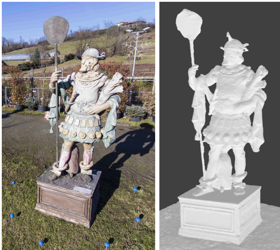
Figure 8. (Left) one of the acquired images from a sculpture by D. Ferretti (Expo 2015, Milan, Italy). Due to its complex shape, this represented a particularly difficult subject to reconstruct with good accuracy. (Right) a view of the reconstructed 3D model of the sculpture.
