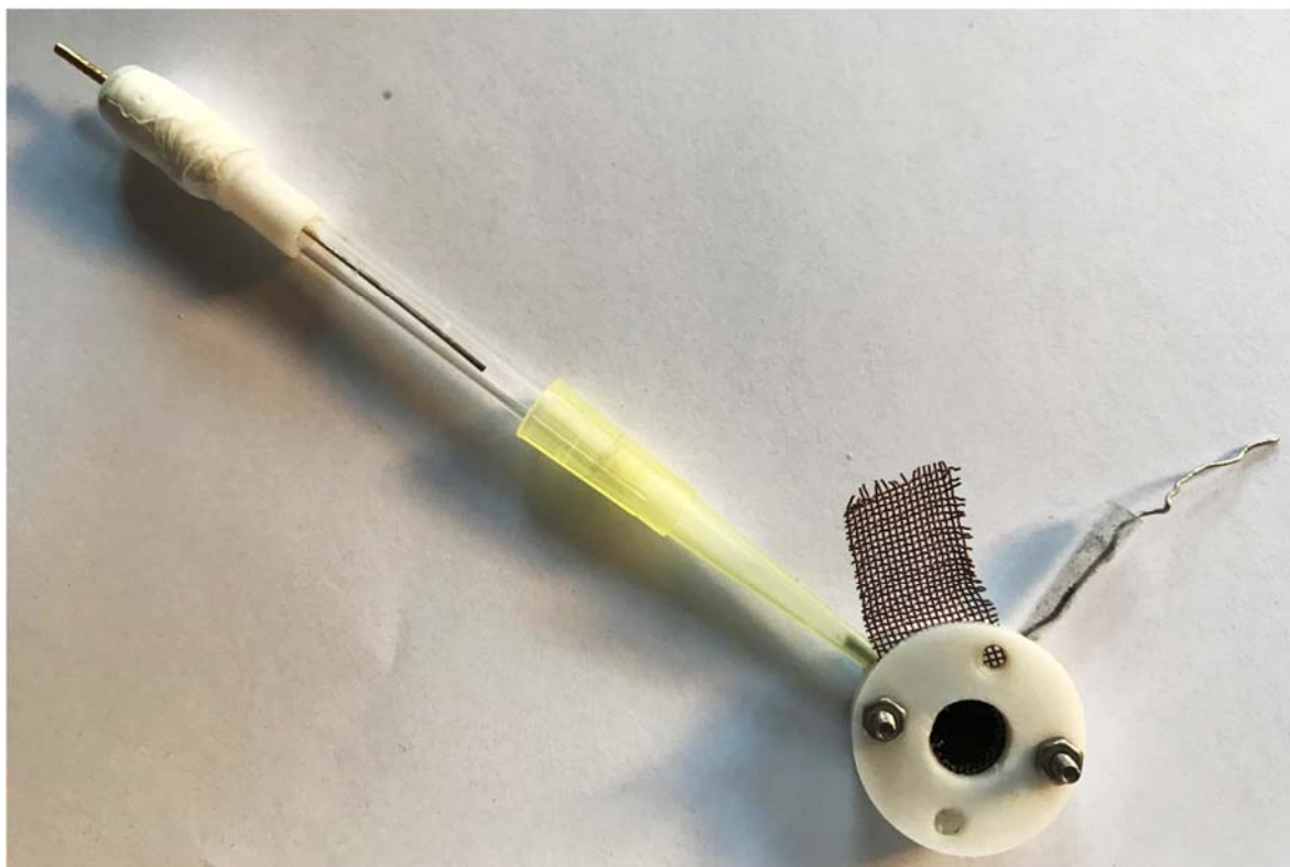
Figure 1. Schematic representation and picture of the spectroelectrochemical cell
