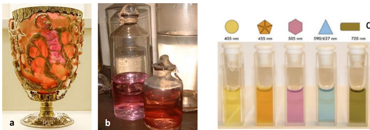
Figure 1.2 (a) The Lycurgus cup (IV century) is the most ancient example of using nanoparticles to change the optical properties of a dielectric. The red colour is due to the plasmonic resonance of the gold nanoparticles embedded in the glass matrix. (b) Suspensions of gold nanoparticles prepared by Michel Faraday (c) Suspensions containing silver nanoparticles with different shapes. The shapes strongly affect the optical absorption of the material.
