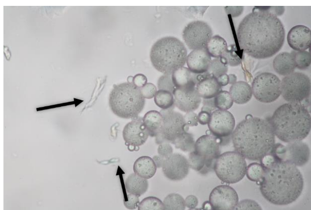
Fig. 3.3 - Light microscopy image of DP microparticles with polymer fibers (indicated by the arrows) formed after the emulsification step.
