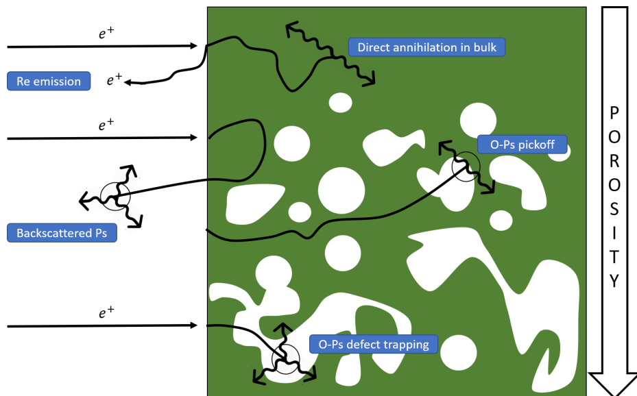
Figure 1.4: Schematic of the possible annihilation channels in porous materials.
